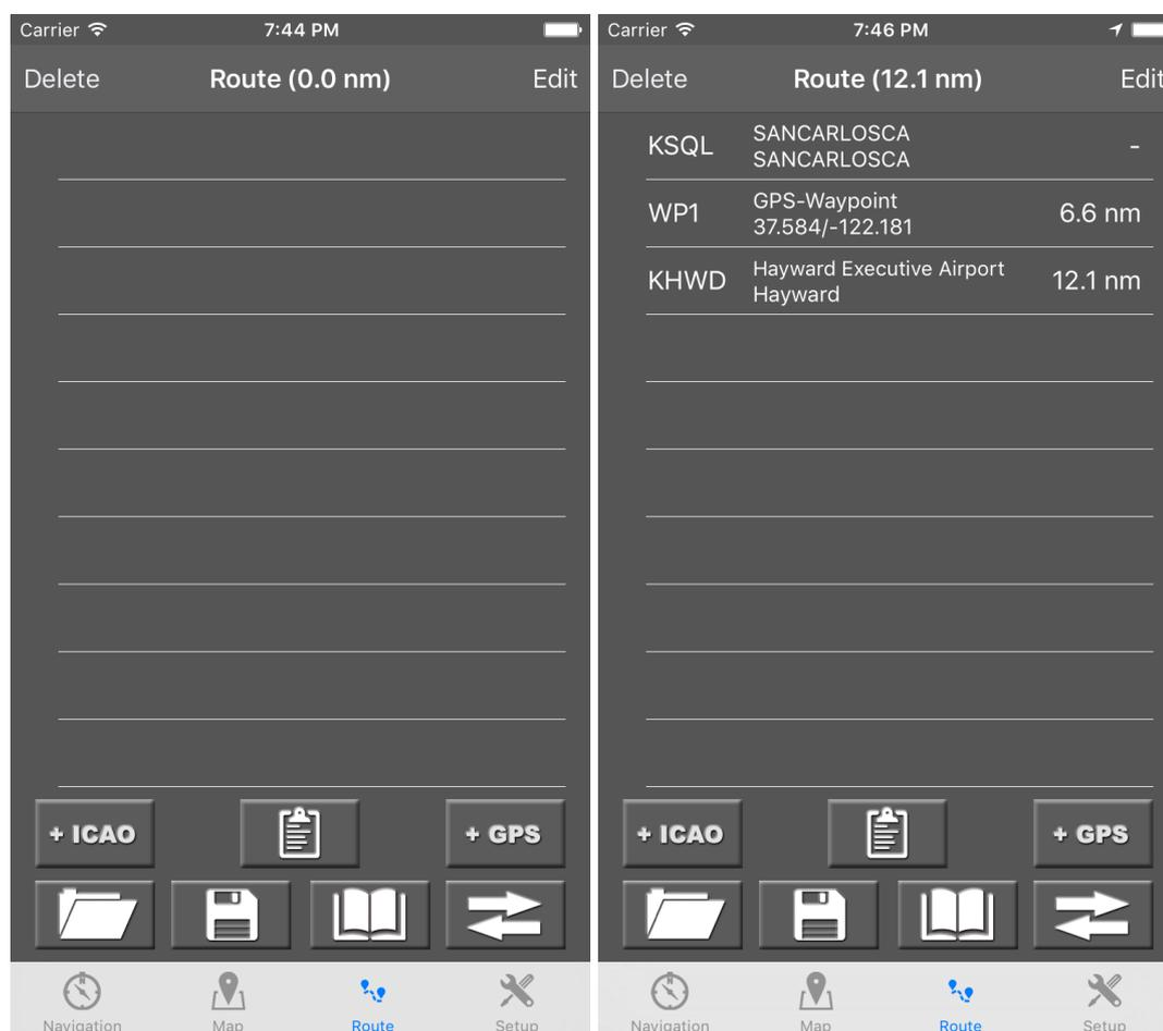
Figure 4.4: Route view. Left hand side: A blank route. Right hand side: A short route from KSQL to KHWD with one free defined GPS-Coordinate.
